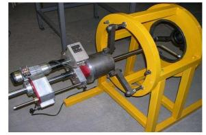
Feed bar motion: Mechanical in accordance with rotation 2 ways and adjustable from 0 to 4 mm/rev
